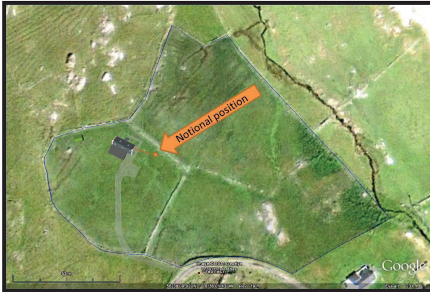
Figure 7: Notional position of Treatment System. Foul drainage will be to a settlement tank and Biorock treatment system; this will drain to a herringbone soakaway.
