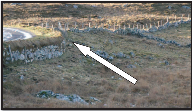
Figure 5: Original position on slope below stone wall, requires a significant infill to achieve a level surface at the intersection with the road
